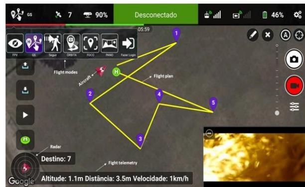
Fig 3: Litchi Android App interface showing flight plan.
