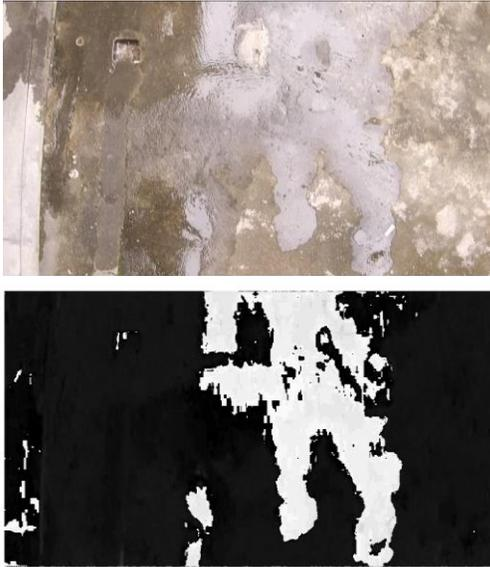
Fig 9: Water puddle converted to HSV.
